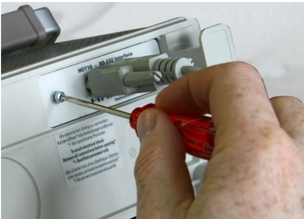
4.1.1 Remove both fastening screws.
