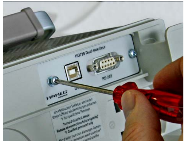
4.2.2 Fit the interface with the fastening screws previously (item 4.1.1) removed.
